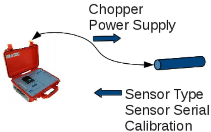
Figure 4 Sensor auto-detection
